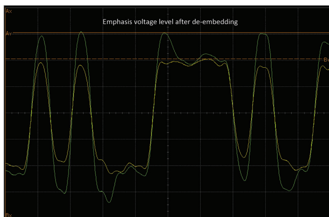
Figure 3. After de-embedding the trace, connector and fixture loss from the yellow waveform, the emphasis voltage level is now visible on the green waveform. You can now verify if the transmitter emphasis meets the SAS-3 requirements
